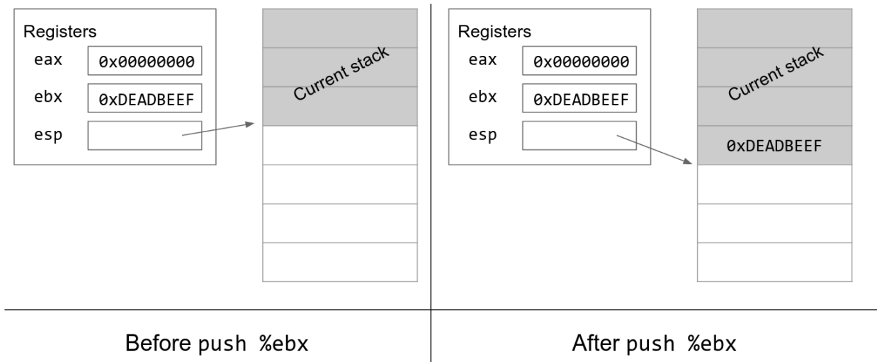
Figure 5: push %ebx decrements esp by 4 and stores the value in the ebx register on the stack.
